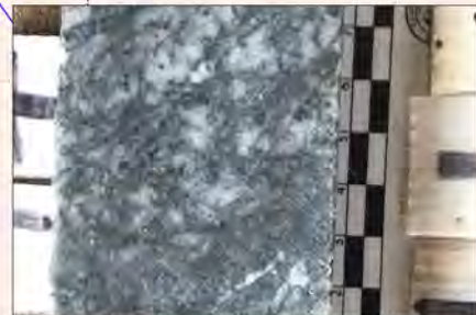
EMD20-111: Eagle-style chlorite and pyrite fractures in granodiorite 94.0m depth ; 1.5m at 3.17 g/t Au
