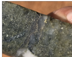
EMD20-102 at 80.0m 1.5m at 18.17 g/t Au Gold associated with silicification and quartz vining
