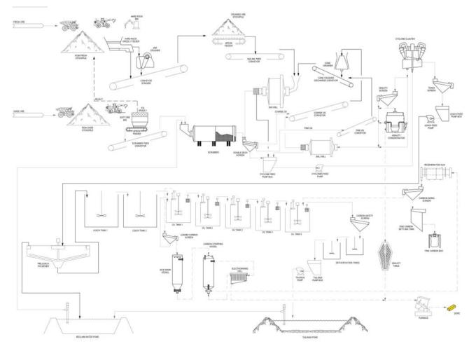
The Phase 2 flowsheet adds the following mechanical equipment to crush and grind transition and fresh rock mill feed down to a size suitable for the CIL process.
