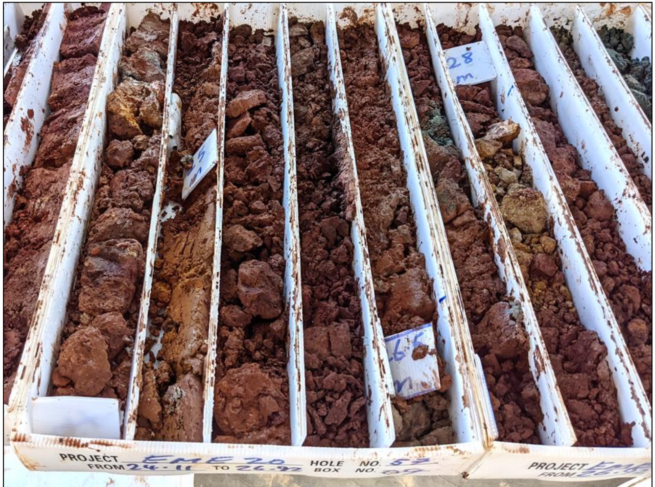
Figure 7-9: Typical mineralized saprolite core from the Salbora area in DDH EME20-57.
